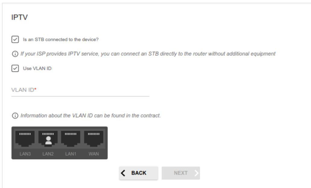
Figure 48. The page for selecting a LAN port to connect an IPTV set-top box.
